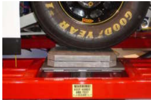
Figure 4 Push Platforms in operation
